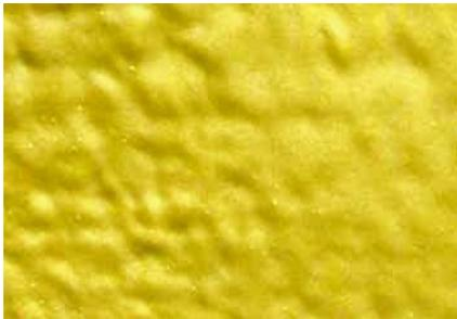
The PTS top coating shown below is an example of pinhole formation as a result of application over an improperly applied and cured sealer coating. The coating also exhibited very weak adhesion.
